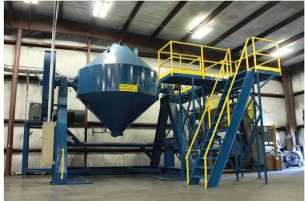
For Sinterite, this project highlights the company's custom in-house design and fabrication capabilities. For Advantage Metals Powders, Inc., installation of this blender increases the company's lot blending capacity from 45,000lbs to 60,000lbs, allowing for a consistent blend in larger lot sizes.
